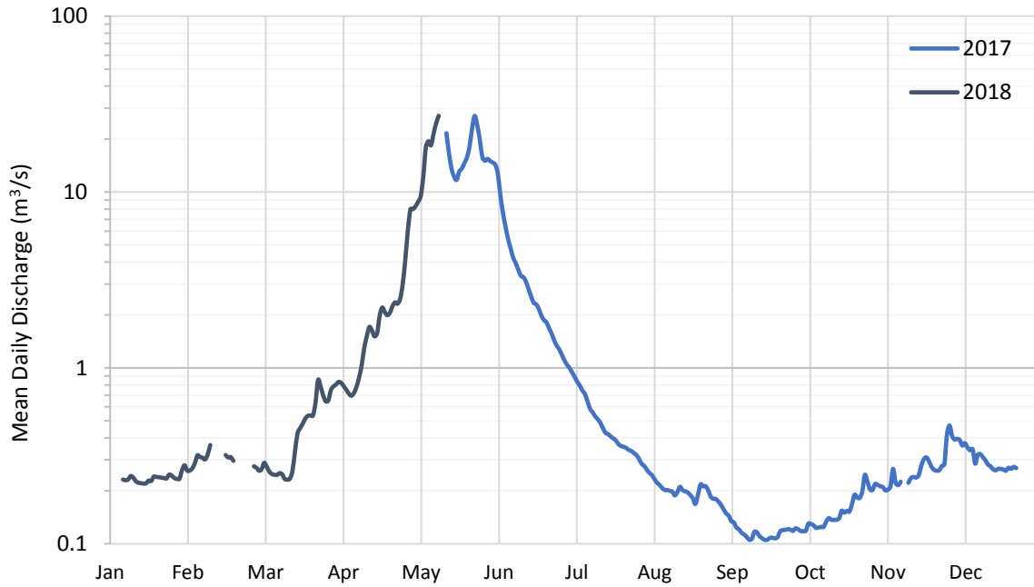
Figure B4-3: Mean daily discharge measured at Whiteman Creek hydrometric station from 2017 to 2018
